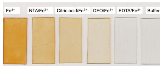
Figure 3. PP-g-PHA films after 24 h of incubation in free Fe 3+ solution, NTA/Fe 3+ (2:1), citric acid/Fe 3+ (2:1), DFO/Fe 3+ (1:1), EDTA/Fe 3+ (1:1), and sodium acetate/imidazole buffer (0.05 M) at pH 5.0.
